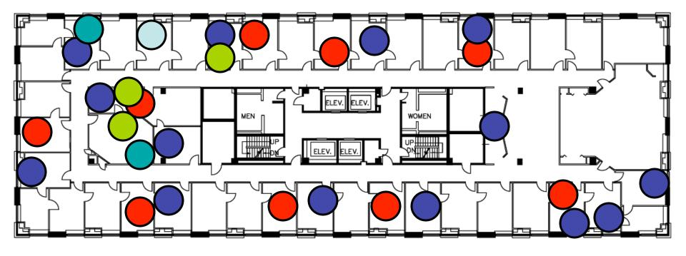
29 PCs with 802.11b radios (fixed transmit power) in 'ad hoc' mode
