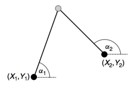
Triangulation from Angular Measurements
