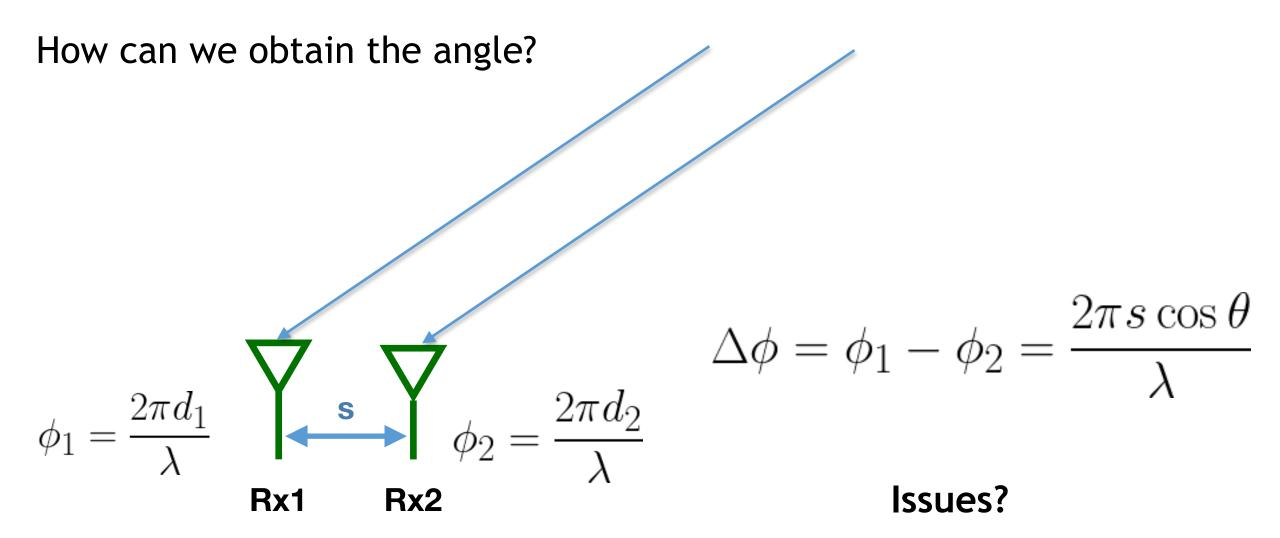
Triangulation from Angular Measurements
