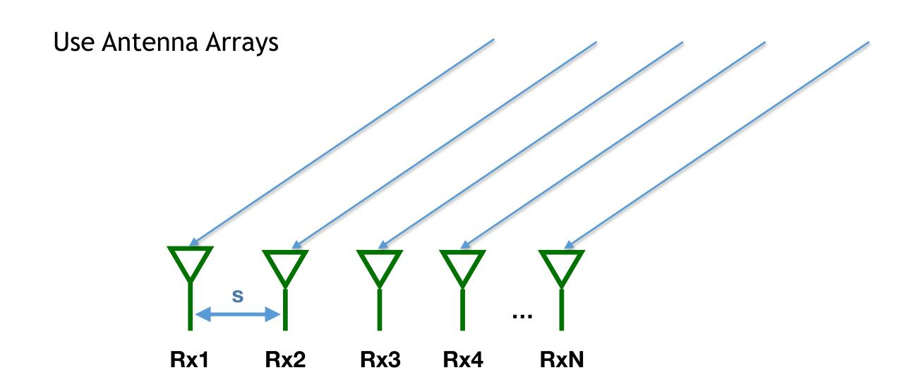
Triangulation from Angular Measurements
